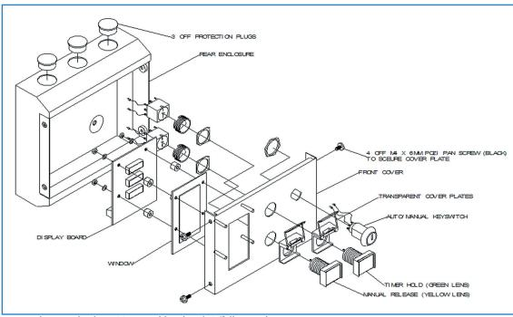
Unit with Manual Release, Timer Hold and Lock Off illustrated
